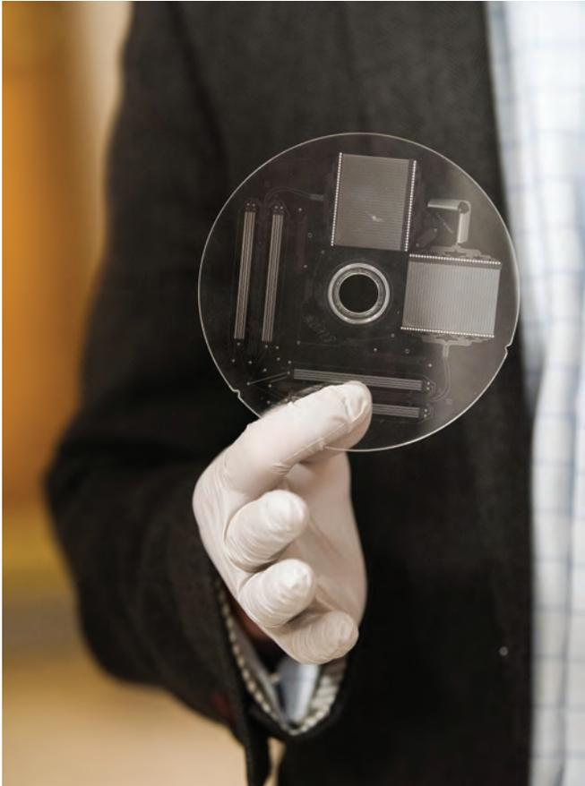
The CTC chip looks like a DVD movie disc but with two tubes attached and a series of tiny channels embedded in it.
